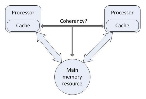
In order to resolve any inconsistencies between cached memory accesses, a *coherency protocol* is required. Various protocols exist to maintain coherency between distributed caches in a multiprocessor system.
